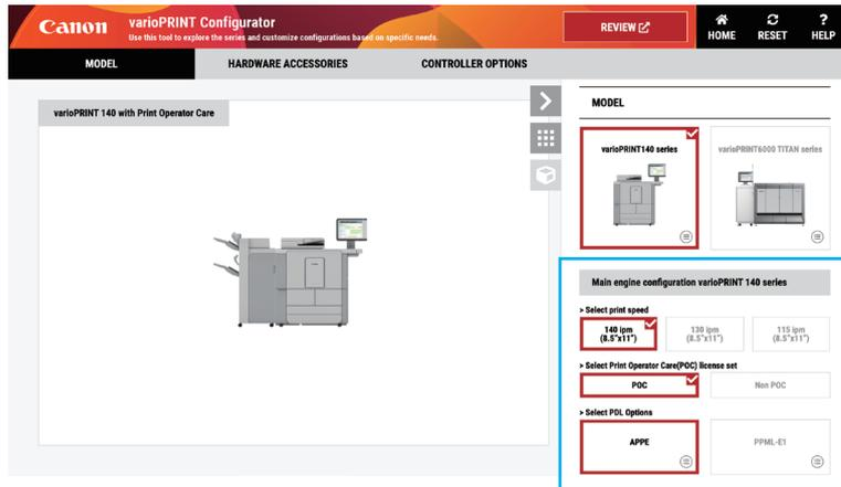
2) Select the main engine configuration and initial configuration settings.
